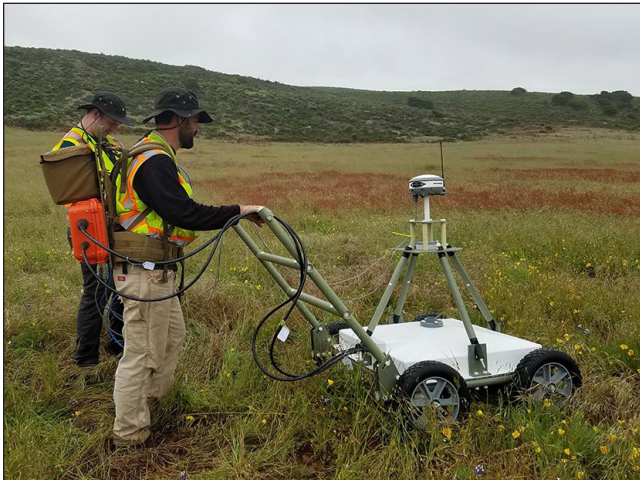
MetalMapper 2x2 static data collection
